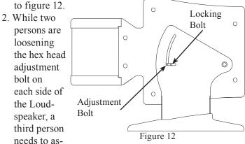
sist by stabilizing the front of the Loudspeaker.
